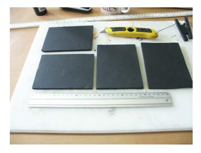
using the Stanley knife and steel rule cut the foam core into four rectangles in this case 14cm x 10cm trying to keep the corners as square as possible
